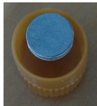
Fig. 1 - Typical sample stub for powder analysis.
